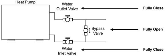
3. Drain the water out of the heat pump by unscrewing the lower union (inlet) and let the water run out.
