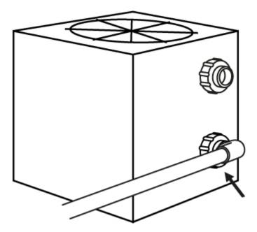
6. Connect the outlet upstream before chlorinator, acid injection or other chemical dosing systems.
