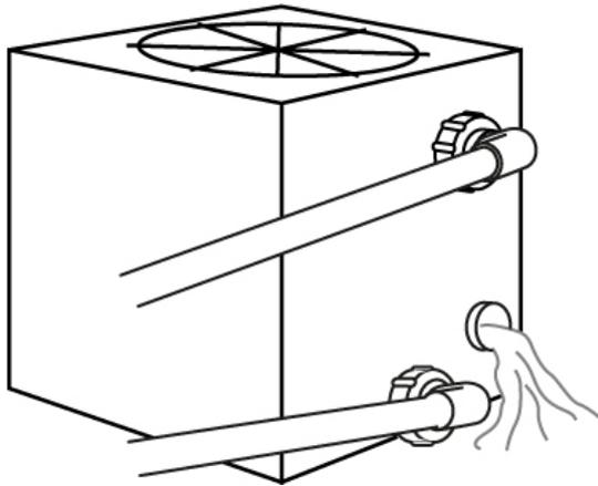
4. Screw the inlet union securely back into place.
