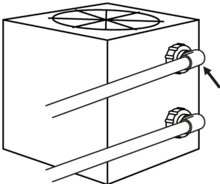
7. Create a flow bypass between the inlet and outlet pipework.
