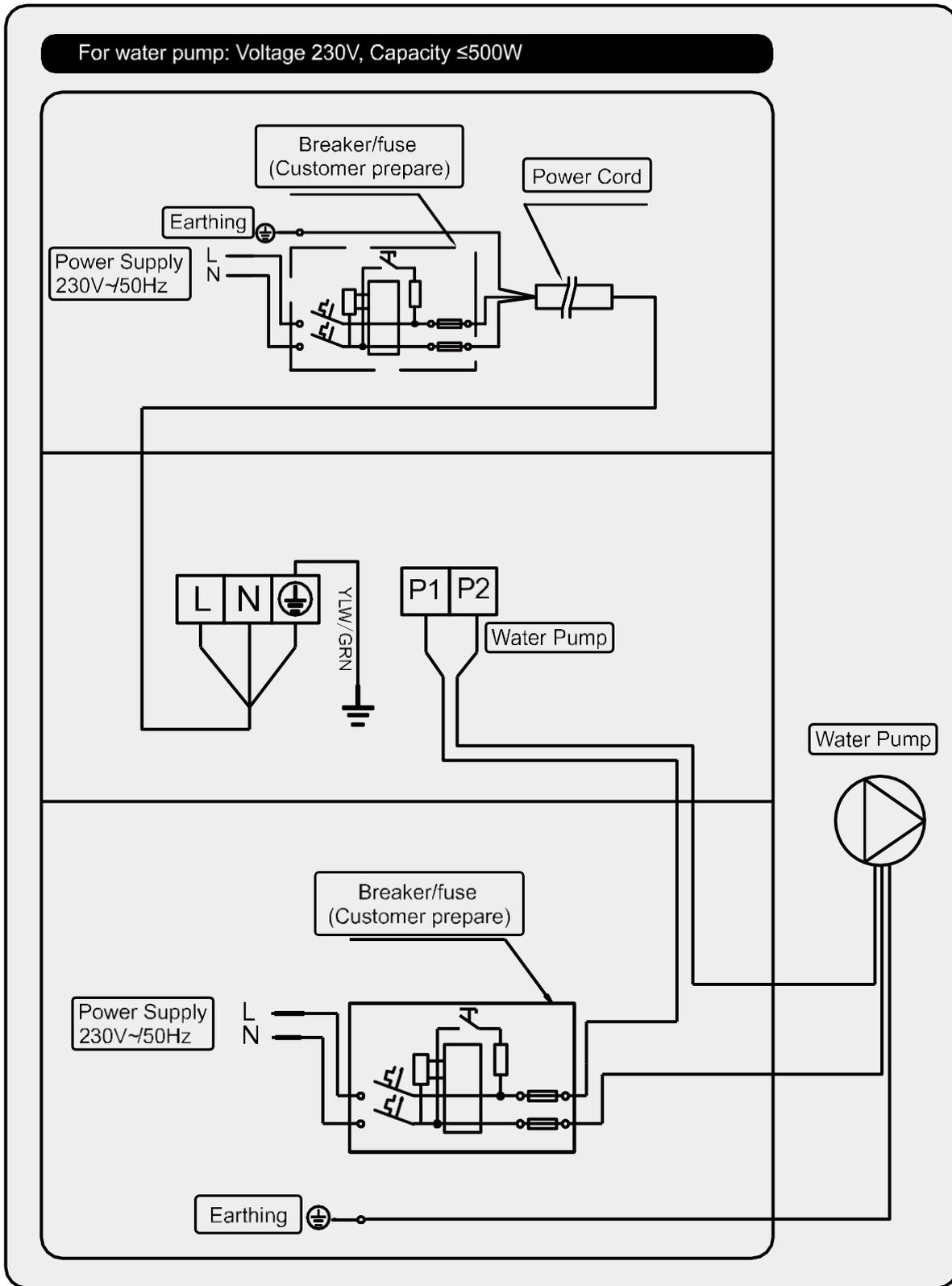
**5.8: WIRING DIAGRAM FOR EXTREME WINTER CONDITIONS: SINGLE PHASE 230V >500W**
