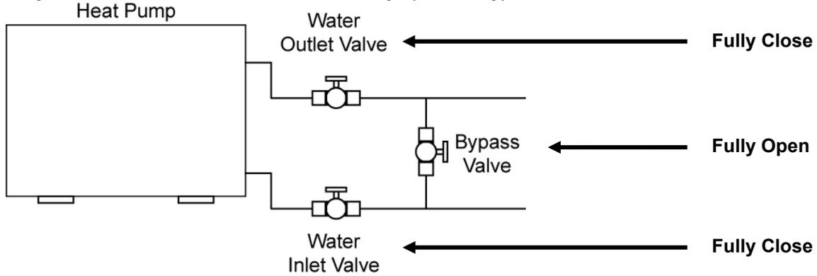
3. Drain the water out of the heat pump by unscrewing the lower union (inlet) and let the water run out.
